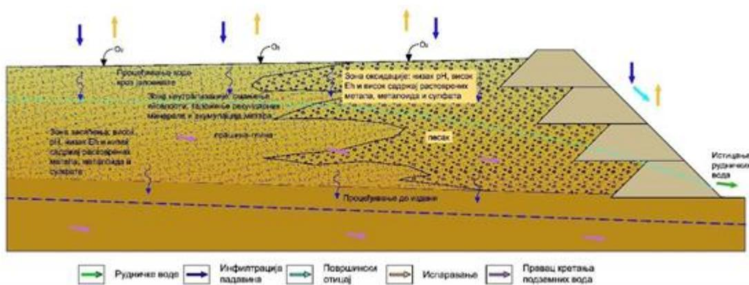
Figure 7: Schematic representation of the formation of drainage waters from the flotation tailings facility<sup>35</sup>
