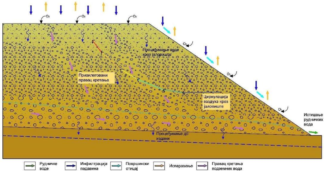
Figure 6: Schematic representation of water and air circulation through the mine tailings facility and the formation of drainage waters<sup>34</sup>
