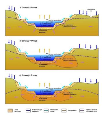
Figure 4: Conceptual model of the impact of surface mines on groundwater and surface water.<sup>32</sup>
