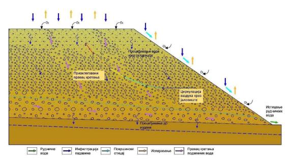
Figure 6: Schematic representation of water and air circulation through the mine tailings facility and the formation of drainage waters<sup>34</sup>
