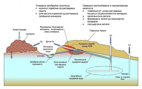
Figure 3: Primary sources and formation of acidic mine waters and pathways through which they reach surface and groundwater<sup>31</sup>
