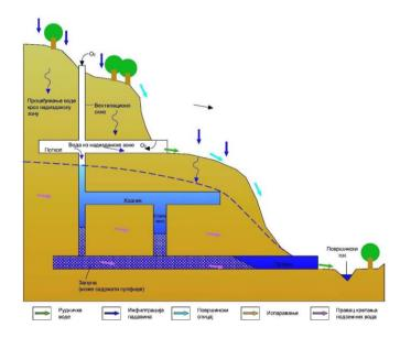
Figure 5: Schematic representation of the formation and discharge of mine waters from abandoned pits<sup>33</sup>
