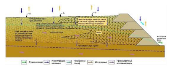
Figure 7: Schematic representation of the formation of drainage waters from the flotation tailings facility<sup>35</sup>
