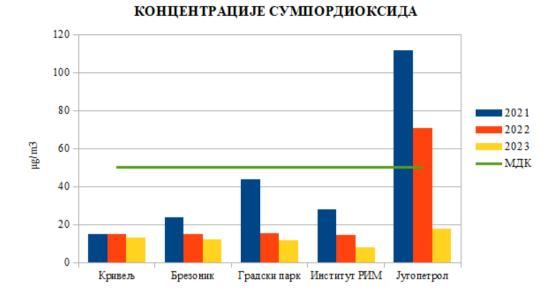
Graph 1: Sulfur Dioxide Concentrations at Measurement Sites in Bor, 2020 - 2023<sup>16</sup>
