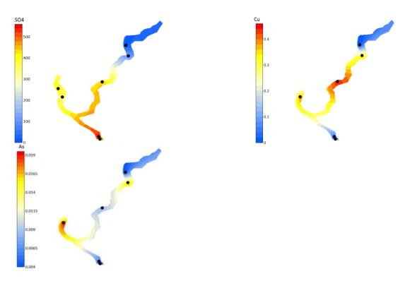
Images 11, 12, and 13: Spatial distribution of arsenic (mg/l), copper (mg/l), and sulfates in water samples from the Small and Large Pek Rivers and the Pek River<sup>38</sup>
