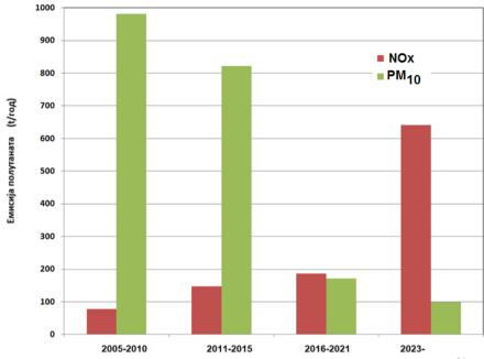
Graph 8: Changes in nitrogen oxide and PM10 emissions from stationary sources in Bor<sup>26</sup>
